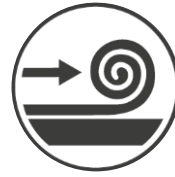
Application of GlasGrid CG/CGL on flat surface and pressure to fresh tack coat
